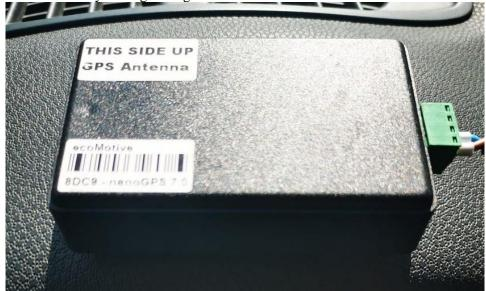
The miniGPS transponder is powered from the vehicle's 12 V battery, or directly using the car's socket (cigarette lighter). Therefore, before presenting yourself at START, you must make sure that your vehicle is equipped with one of the following solutions:
